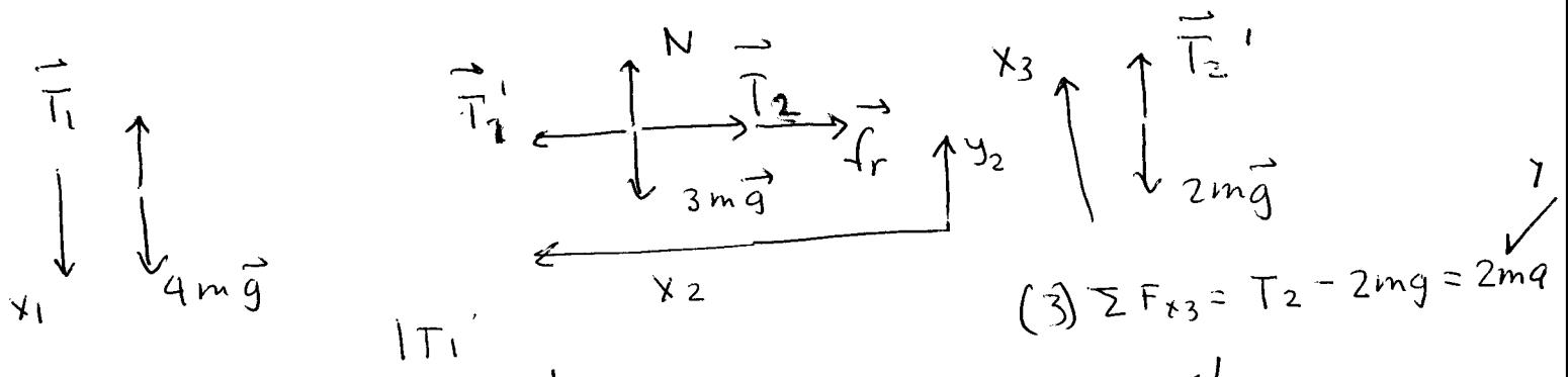
$$(1) \sum F_{x_1} = 4mg - T_1 = 4ma \quad (2) \sum F_{x_2} = T_1 - T_2 - fr = 3ma \quad (3) \sum F_{x_3} = T_2 - 2mg = 2ma$$
