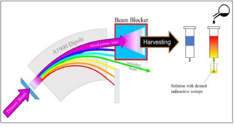
Figure 1. Graphic showing how isotopes will be produced and harvested from the FRIB facility at MSU with unused beam. Note that the secondary beam is the beam in which experimenters using the facility would be interested.
