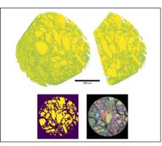
Figure 2. Computed Tomography (CT) image (top) of mock HE, courtesy of B.M. Patterson and J.D. Yeager (LANL), with watershed segmentation (bottom) by C.G. Becker and A.J. Clarke (Colorado School of Mines).
