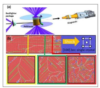
Figure 2. (a) Experimental setup at the NIF. Hohlraum is illuminated by 192 beams, and backlighter illuminates target for side-on radiography. (b) Molecular dynamics simulation of iron subjected to 55 GPa shock. The top image shows shock wave passing through single crystal bcc iron. The bottom image shows evolution of nanostructure as shock passes through. Colors represent different phases: blue = BCC, green = FCC, red = HCP, white = unidentified.
