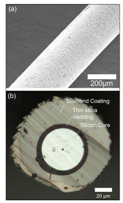
Figure 2. (a) Scanning electron microscope image of diamond encapsulated silicon fiber showing homogeneous morphology. (b) Cross section of a 50 micron silicon fiber after polishing in an ion mill. The fiber is clad in a thin layer of silica and coated in diamond.
