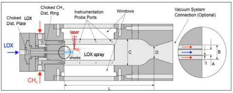
Figure 1. Computer-aided design schematics of the INSIEME experimental rocket-combustor geometry (courtesy of Carson Slabaugh, Purdue University).
