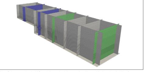
Figure 2. A computational grid for turbulence simulations produced by a grid-adaptation algorithm (i.e., without user input).
