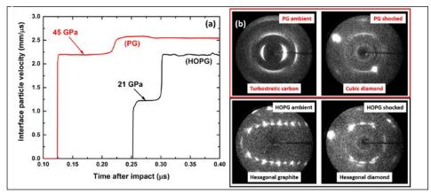
Figure 1. (a) Wave profiles and (b) XRD images from PG (red) and HOPG (black). Transformation stresses are labeled in (a), and the ambient and high-stress crystal structures are labeled in (b). Data in (a) and (b) are from Volz et al., J. Appl. Phys. 125, 245902 (2019), and Volz et al., Phys. Rev. B 101, 224109 (2020), respectively.
