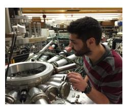
Figure 1. Charged-particle time-of-flight chamber used for charged-particle evaporation spectrum measurements.
