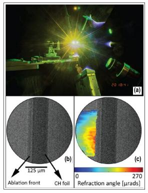
Figure 2. (a) Visible camera image of the EP-TXD diagnostic in the Irradiated Foil campaign. (b) Raw Moiré image of the 125  $\mu$ m CH irradiated foil (150 J, 1 ns) obtained through TXD at 5 ns. (c) Refraction angle 2D map retrieved through TXD methods.
