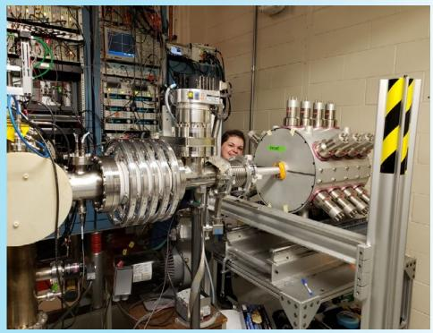
Lewis setting up the Summing Nal (SuN) detector for an experiment at the NSCL.
