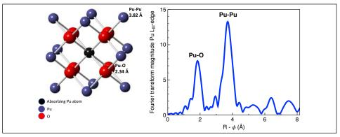
Figure 1. Extended X-ray absorption fine structure (EXAFS) spectra of a PuO<sub>2</sub> sample that was corroded from Pu metal (left) showing peaks that correspond to the Pu-O and Pu-Pu shells of the PuO<sub>2</sub> structure on the right.
