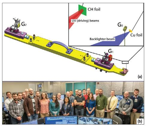
Figure 1. (a) EP-TXD diagnostic platform. b) Johns Hopkins researchers and the scientific team that participated in the FY20 EP-TXD Irradiated Foils campaign.
