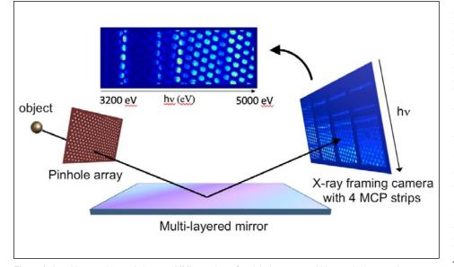
Figure 1. A multi-monochromatic imager, MMI, consists of a pinhole-array, multi-layered mirror, and microchannel plate (MCP), which records hundreds of object images with a horizontal photon-energy axis.
