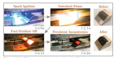
Figure 1. Mach 2.7 supersonic combustion with carbon fiber insert: an example prediction target in the Illinois ACT-II arc-driven supersonic combustion tunnel (designed and operated by CEESD co-PI Tonghun Lee with Air Force Office of Scientific Research AFOSR funding). There is obvious degradation of the model carbon fiber composite, here a surrogate for more practical engineering materials.
