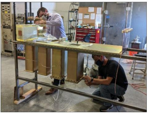
Figure 2. Graduate student Travis Bejines and IAC Engineer Brian Berls assembling the 4-Brick Cinco generator. This device, capable of 320 kA, will allow the validation of all key components, a necessary step before building larger Cinco devices with ramp compression loads.
