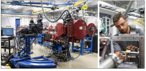
Figure 1. Impact Facilities: Two-stage gun and X-ray detectors (left) and mounting a target (right).
