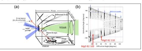
Figure 1. (a) Experiment geometry of the PXRDIP diagnostic at the OMEGA-60 laser system. (b) *In situ* X-ray diffraction pattern of ramp-compressed MgO projected into phi—d–spacing coordinates. Observed peaks demonstrate formation of the high pressure B2 phase of MgO.
