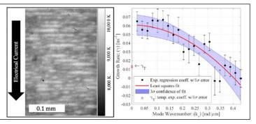
Figure 1. Left: ETI perturbations are seen in the aluminum-6061 surface temperature (from a 3-µm/3.5-ns-FWHM-resolution image). Right: ETI exponential growth rate vs perturbation wavenumber.
