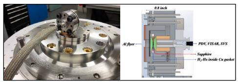
Figure 1. (Left) Assembled pre-compression cell in a stripline geometry for a Z experiment. (Right) Schematic of a pre-compression cell (2 inches wide and 0.8 inch tall). The fluid mixture of hydrogen-helium is captured inside the copper gasket placed in between two sapphire anvils.
