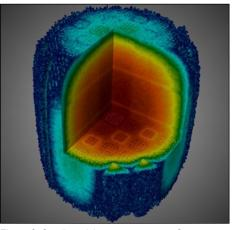
Figure 2. Small modular reactor neutron flux contours from Shift.
