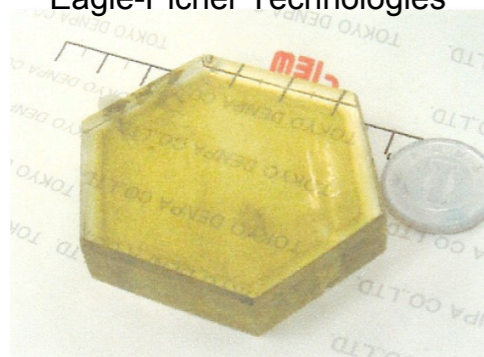
Figure 2. Photograph of a 2 inch ZnO single crystal. Maeda et. al. , Semicond. Sci. Technol. 20 (2005) S49-S54
