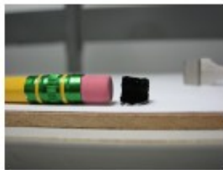
Longest nanotubes by CVD: 7 mm
