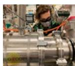
Chad Ummel couples the GODDESS ionization chamber to the scattering chamber containing the Oak Ridge Rutgers University Barrel Array (ORRUBA) in preparation for an experiment at the National Superconducting Cyclotron Laboratory.
