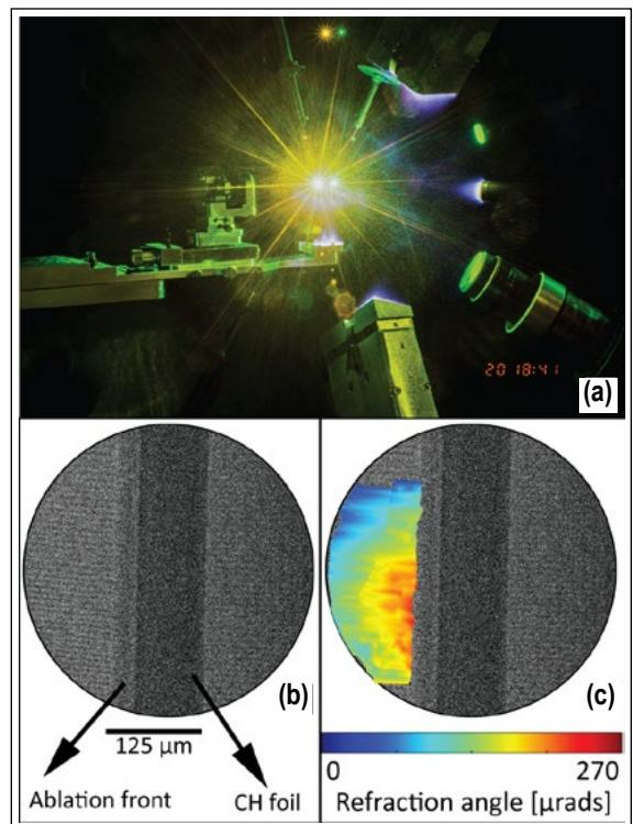
Figure 2. (a) Visible camera image of the EP-TXD diagnostic in the Irradiated Foil campaign. (b) Raw Moiré image of the 125  $\mu\text{m}$  CH irradiated foil (150 J, 1 ns) obtained through TXD at 5 ns. (c) Refraction angle 2D map retrieved through TXD methods.
