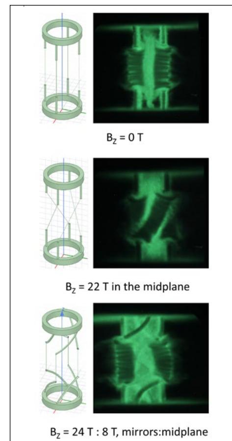
Figure 3. XUV images are shown together with the three specified load configurations when driven by 1 MA from COBRA.
