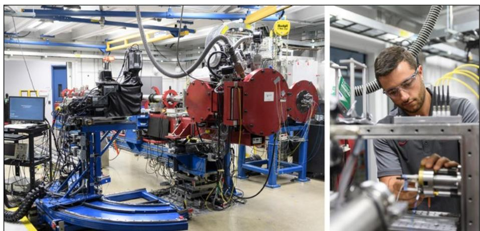
Figure 1. Impact Facilities: Two-stage gun and X-ray detectors (left) and mounting a target (right).
