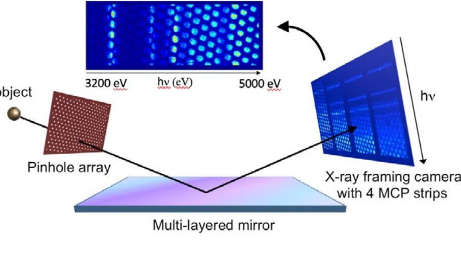
Figure 1. A multi-monochromatic imager, MMI, consists of a pinhole-array, multi-layered mirror, and microchannel plate (MCP), which records hundreds of object images with a horizontal photon-energy axis.
