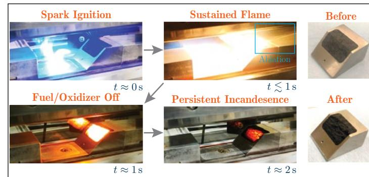
Figure 1. Mach 2.7 supersonic combustion with carbon fiber insert: an example prediction target in the Illinois ACT-II arc-driven supersonic combustion tunnel (designed and operated by CEESD co-PI Tonghun Lee with Air Force Office of Scientific Research AFOSR funding). There is obvious degradation of the model carbon fiber composite, here a surrogate for more practical engineering materials.
