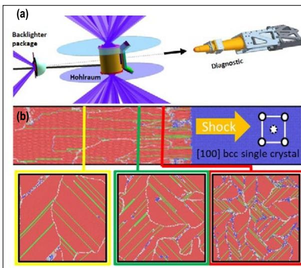
Figure 2. (a) Experimental setup at the NIF. Hohlraum is illuminated by 192 beams, and backscatter illuminates target for side-on radiography. (b) Molecular dynamics simulation of iron subjected to 55 GPa shock. The top image shows shock wave passing through single crystal bcc iron. The bottom image shows evolution of nanostructure as shock passes through. Colors represent different phases: blue = BCC, green = FCC, red = HCP, white = unidentified.
