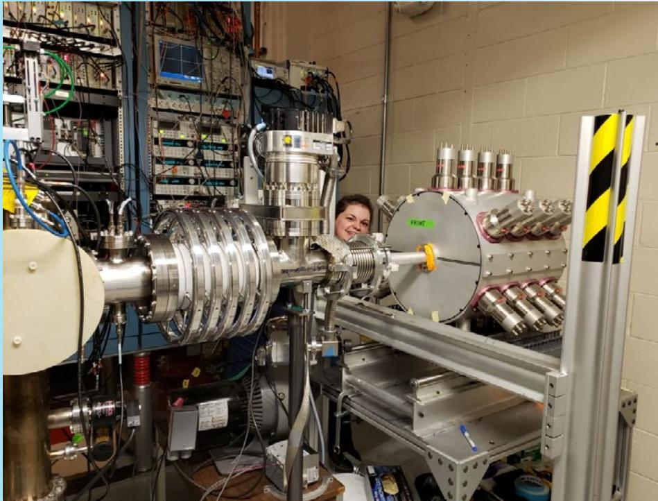
Lewis setting up the Summing NaI (SuN) detector for an experiment at the NSCL.
