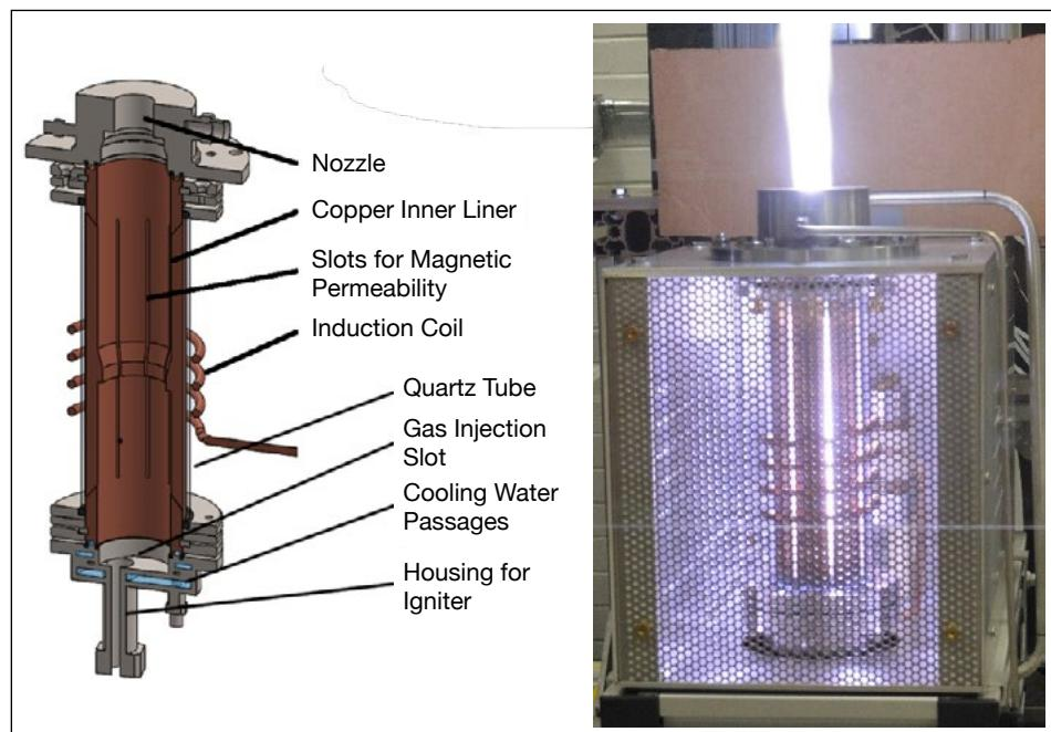
Figure 1. University of Texas plasma torch overview: cross-section of the plasma chamber (left) and torch in operation (right).
