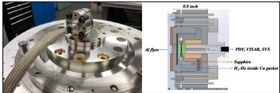
Figure 1. (Left) Assembled pre-compression cell in a stripline geometry for a Z experiment. (Right) Schematic of a pre-compression cell (2 inches wide and 0.8 inch tall). The fluid mixture of hydrogen-helium is captured inside the copper gasket placed in between two sapphire anvils.
