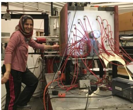
Figure 2. The HeBGB neutron detector for ( $\alpha, n$ ) measurements.
