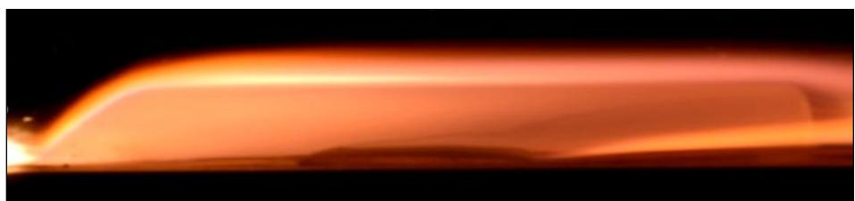
Figure 1. Slab motor experiment showing the burning of paraffin wax fuel used in hybrid rockets.
