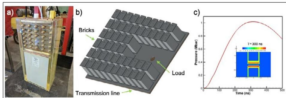
Figure 1. (a) Cinco building block, the 100 kA brick. (b) 50-brick Cinco generator with strip-line quasi-isentropic compression load. (c) Performance of fully configured Cinco showing the compression of copper to 1 Mbar (100 GPa).
