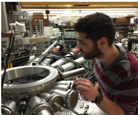
Figure 1. Charged-particle time-of-flight chamber used for charged-particle evaporation spectrum measurements.
