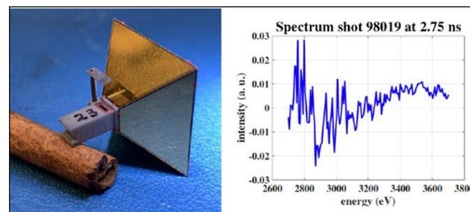
Figure 3. A target for the Omega Laser Facility (left) and a preliminary absorption spectrum (right). Image credit: Sallee Klein and Heath LeFevre, University of Michigan
