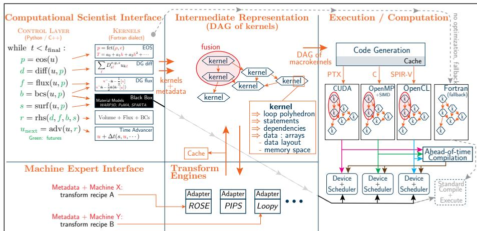
Figure 2. The MIRGE computer science framework, designed to balance usability (with python-based control layer) against portability, which is facilitated by the abstractions of the intermediate representation and existing hardware-targeted code-generation tools.
