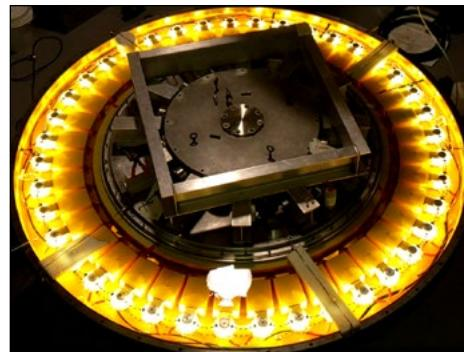
Figure 2. LTD Pulsed Power Machine MAIZE at the University of Michigan shown firing after being upgraded with 40 new switches.
