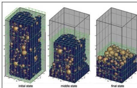
Figure 1. Simulation of particle gravity deposition with hybrid OpenMP-MPI Discrete Element Method (DEM) code ParaEllip3d. Maximum to minimum particle diameter ratio = 10.
