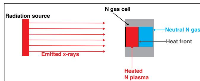
Figure 2. Schematic of a photoionization front experiment where an x-ray source is incident on a nitrogen gas cell. Image Credit: Heath LeFevre, University of Michigan
