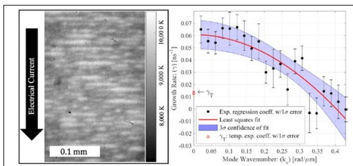
Figure 1. Left: ETI perturbations are seen in the aluminum-6061 surface temperature (from a 3-μm/3.5-ns-FWHM-resolution image). Right: ETI exponential growth rate vs perturbation wavenumber.
