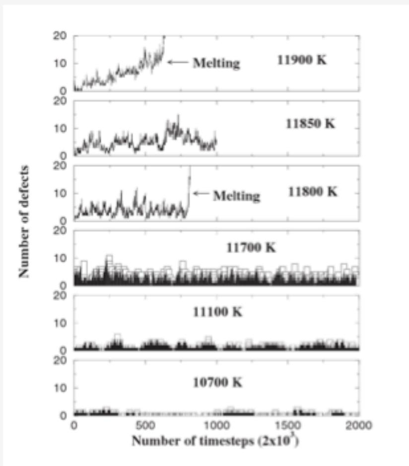
The number of defects sharply increases on melting (instead of accumulating gradually). This suggests a mechanism of melting not due to the nucleation of liquid, but due to the generation of percolating defects on the system.
