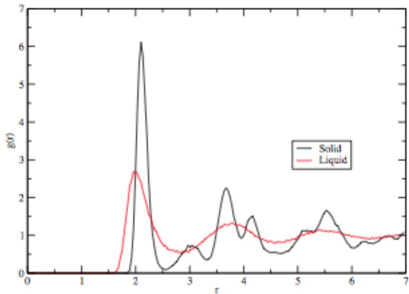
First thing one would try is just heat the solid and see when it changes in terms of structure or transport properties. However, this gives the wrong  $T_m$  because of overheating.
